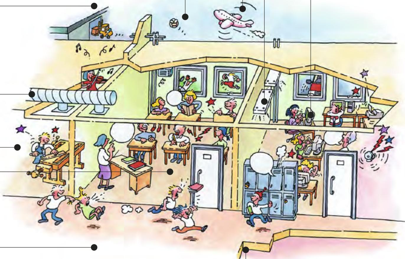
Noise due to footfall arises very frequently, for example with wooden floors. If the load-bearing structures are poorly insulated, the sound can also easily penetrate rooms located below.
